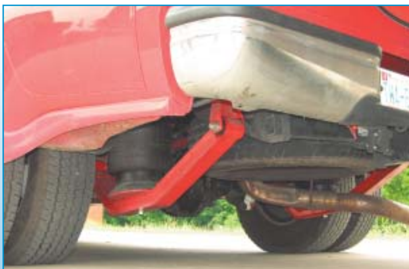
The company's latest prototype product is rear air-bag suspension kits for 1-ton pickups.
